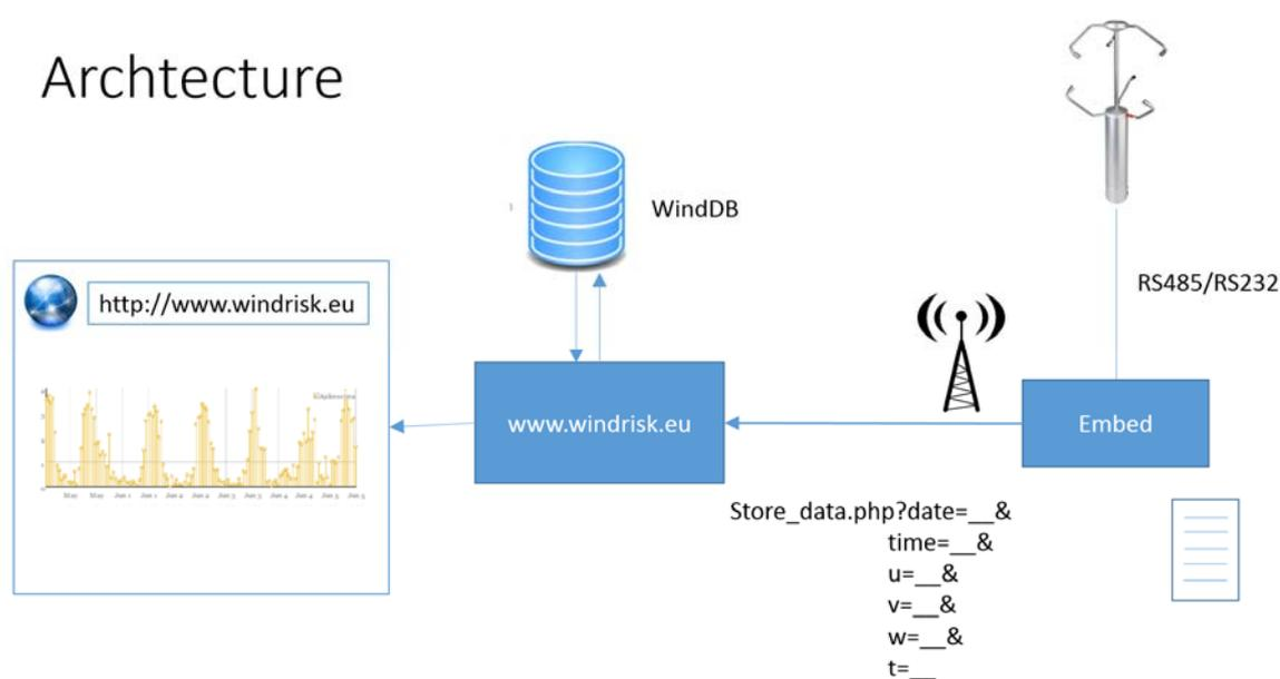
Figure 7: Wind measurement system architecture
