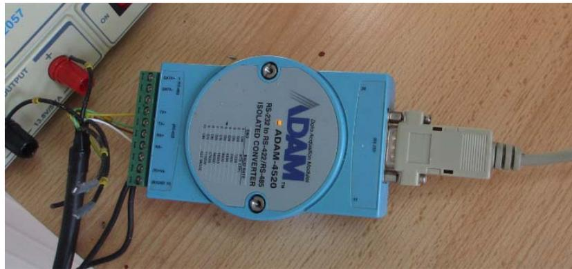
Figure 3: Connector for 3D ultrasonic anemometer
