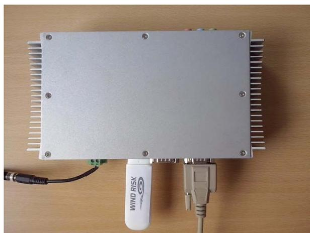
Figure 4: Embedded Linux computer for the streaming of data measurement
